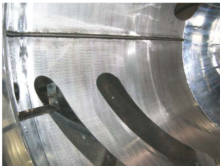
Interior of VHC-66L 1000L Coating Pan Showing mixing baffles, anti-slide baffles, and slotted perforations
