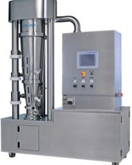
VFC-LAB 1 0.6L to 4L Bowl Capacities - For Top Spray Granulation, Drying, Wurster
